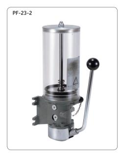
Single- and dual-circuit piston pumps are designed for the operation of centralized lubrication systems with progressive feeders on small and medium-size machines and equipment.
